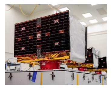
Aerospacelab has designed the Versatile-Satellite Platform (VSP), a flight-proven satellite platform ready to support a variety of LEO missions. With a standardized modular core design, the VSP is quickly adapted for a wide range of payloads, including optical imagery, radio frequency detection instruments, telecom services, space domain awareness and missile defense.
